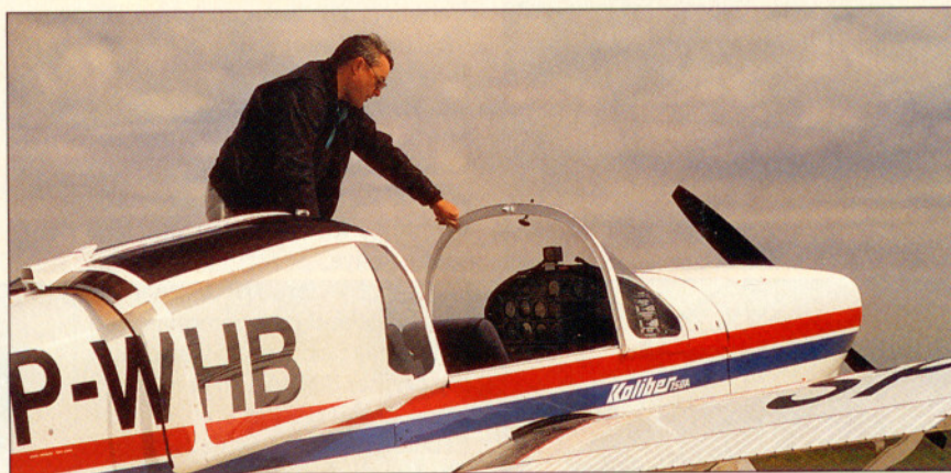
The Koliber's slats automatically extend at slow airspeeds and make for docile stalls. At or below 92 knots, the canopy can be fully opened—but say goodbye to loose objects.
